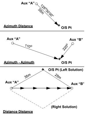
Figure 2-12: Offset Methods (Graphical)
